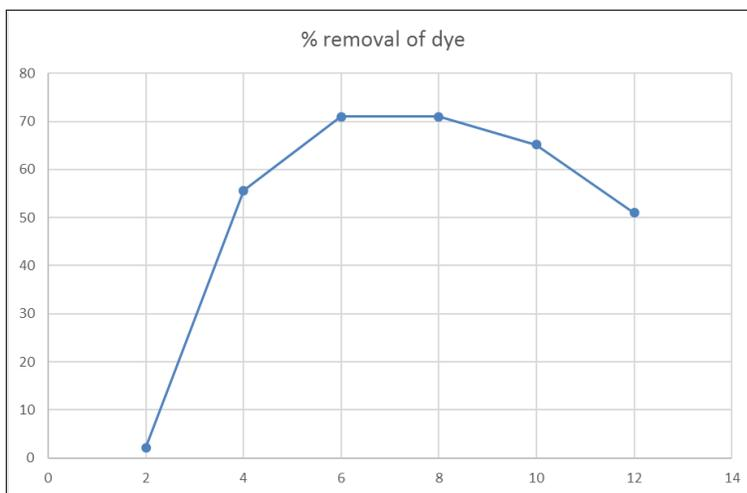
**Fig 5:** Removal of dye Varying of pH by keeping constant dye concentration and coagulant dosage
