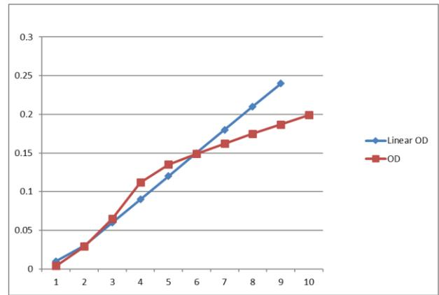
Fig 1: Calibration curve for Methyl Orange
