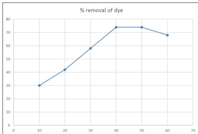
**Fig 6:** Removal of dye varying of contact time by keeping constant dye concentration and coagulant dosage
