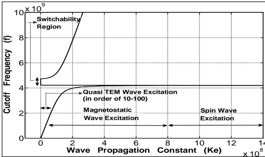
Fig 2: Dispersion curve (f Vs.  $K_e$ ) of LiTiMg for incident plane wave perpendicular to biased substrate, magnetized by 1500 Oe magnetic field in the X band.
