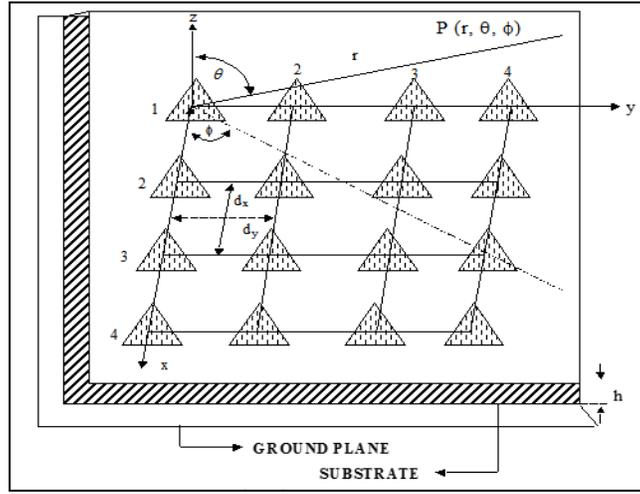
Fig 1: Geometry of 4 × 4 array microstrip triangular patch antenna
