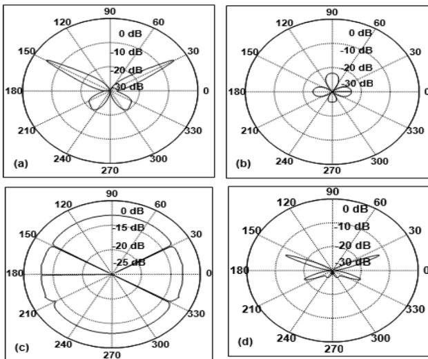
**Fig 3:** Comparison of RHCP radiation patterns of triangular patch microstrip array antenna for external biasing field (a)  $H_0 = 0$  Oe with TR-duroid substrate, (b)  $H_0 = 0$  Oe with Silicon substrate, (c)  $H_0 = 0$  Oe with Ferrite substrate, (d)  $H_0 = 1500$  Oe with Ferrite substrate.
