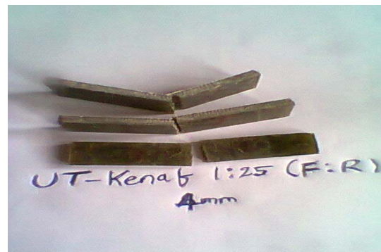
Fig 8: Flexure Tested specimen of untreated kenaf fiber at 4mm
