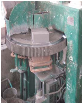
Fig 15: Manufacture Of Bricks Using Semi-Automatic Fly ash Making Machine
