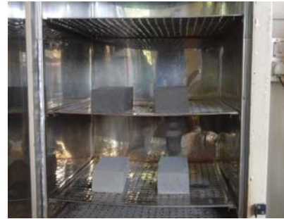
Fig 13: Dry Hot Oven Curing
