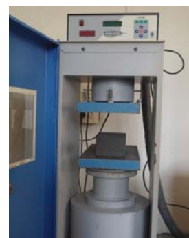
Fig 14: Compression Test in ACTM
