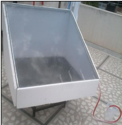
Fig 2: Experimental set up of simple SS
