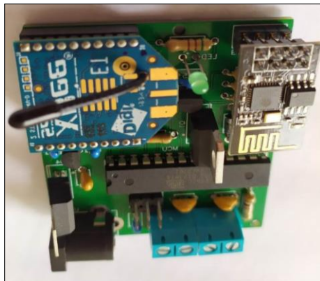
Fig 2: Implemented Master Node PCB
