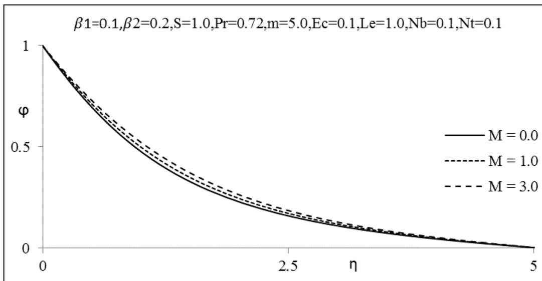
Fig 1(d): Concentration profiles for various values of M
