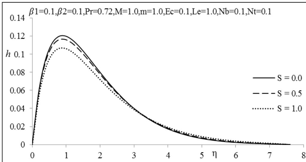
**Fig 5(b):** Transverse velocity profiles for various values of  $S$
