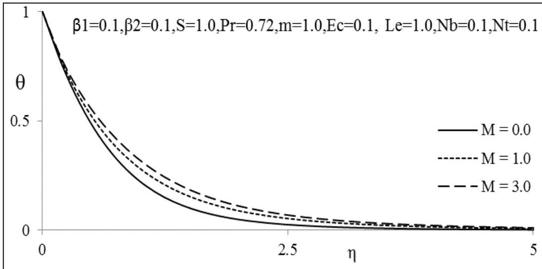
Fig 1(c): Temperature profiles for various values of M
