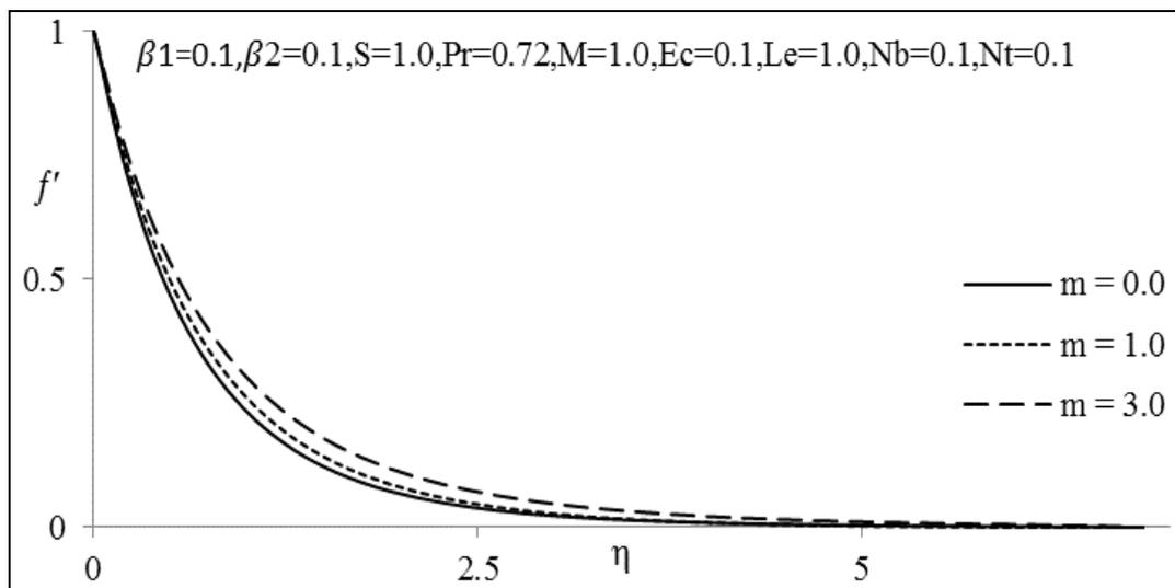
Fig 2(a): The variation axial velocity profiles with increasing values of m
