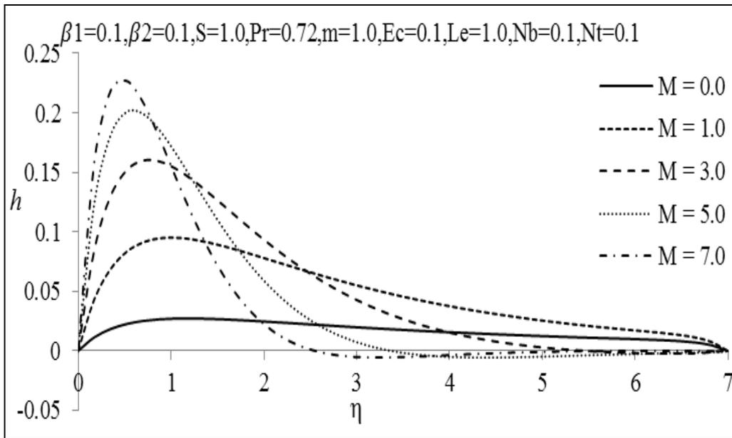
Fig 1(b): Transverse velocity profiles for various values of M
