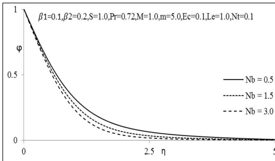
Fig 8(b): Concentration profiles for various values of  $Nb$
