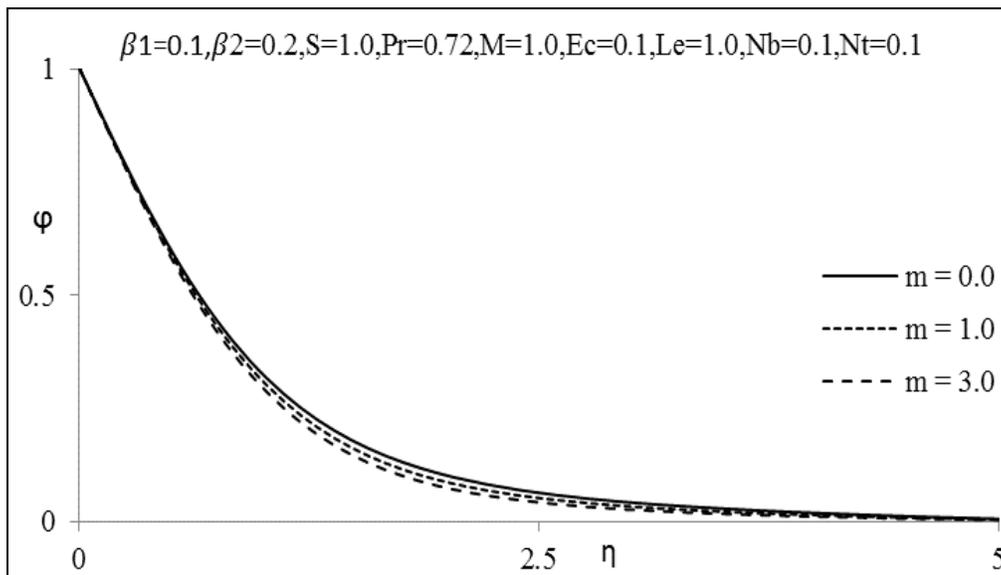
Fig 2(d): Concentration profiles for various values of m
