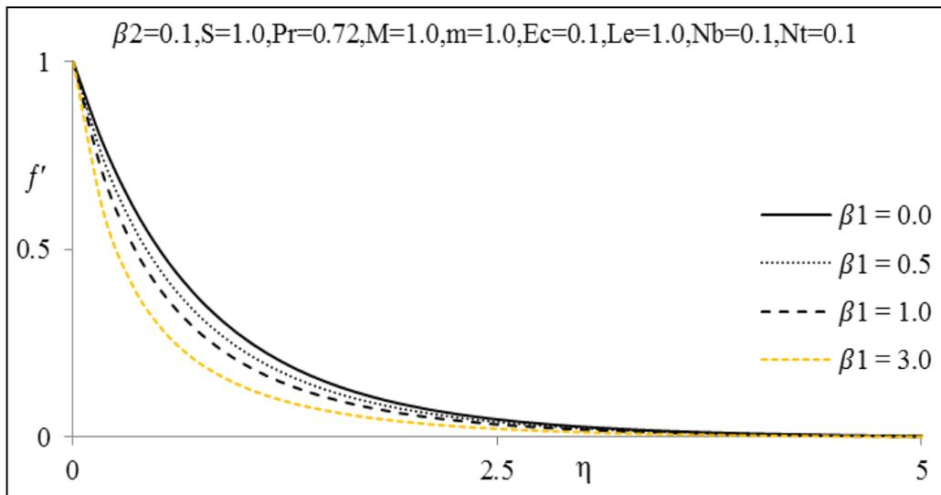
**Fig 4(a):** The variation axial velocity profiles with increasing values of  $\beta_1$
