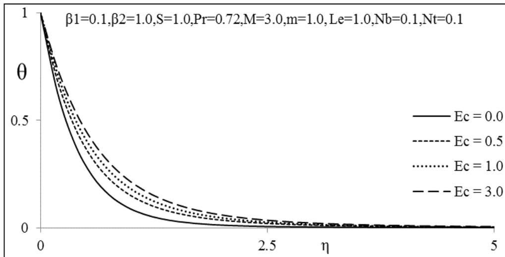
Fig (c): Temperature profiles for various values of  $Ec$
