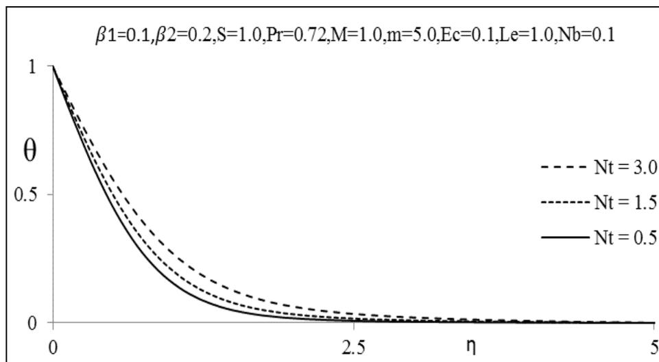
**Fig 7(a):** Temperature profile for various values of  $Nt$
