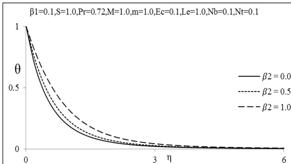
**Fig 6(b):** Temperature profiles for various values of  $\beta_2$
