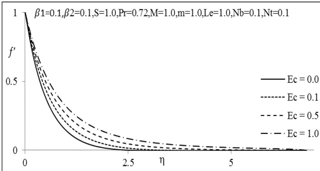
Fig 3(a): The variation axial velocity profiles with increasing values of  $Ec$
