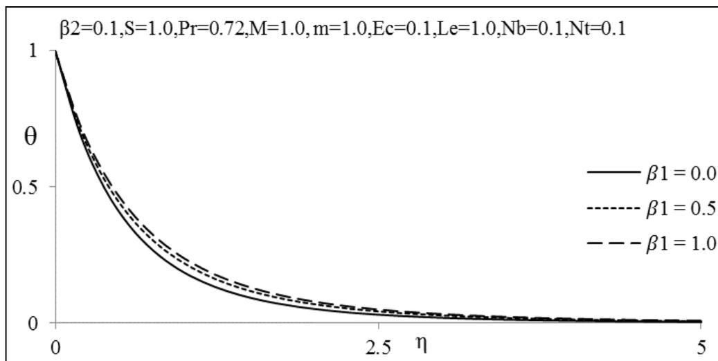
**Fig 4(c):** Temperature profiles for various values of  $\beta_1$
