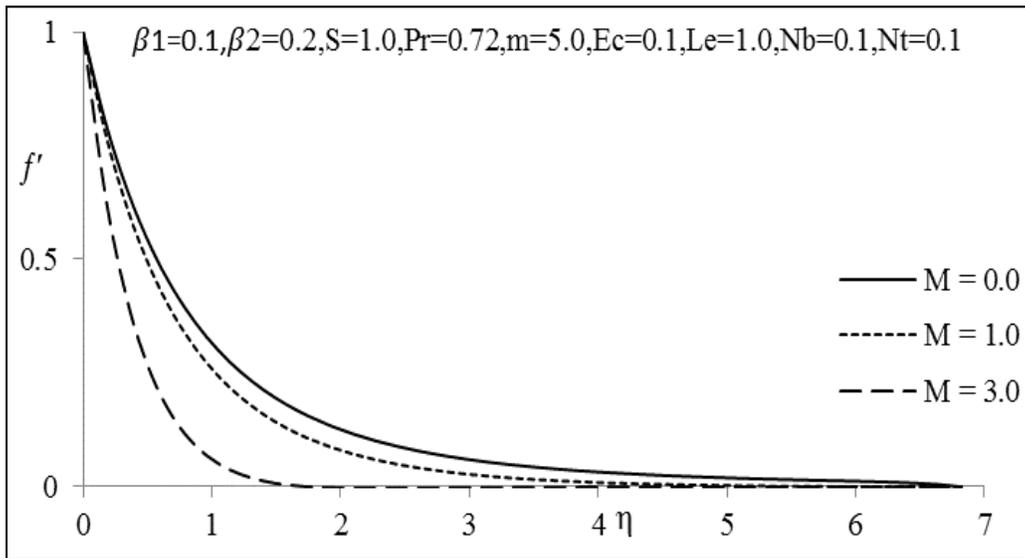
Fig 1(a): The variation axial velocity profiles with increasing values of M
