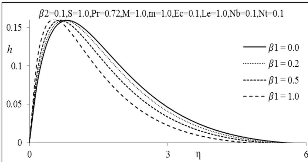
**Fig 4(b):** Transverse velocity profiles for various values of  $\beta_1$
