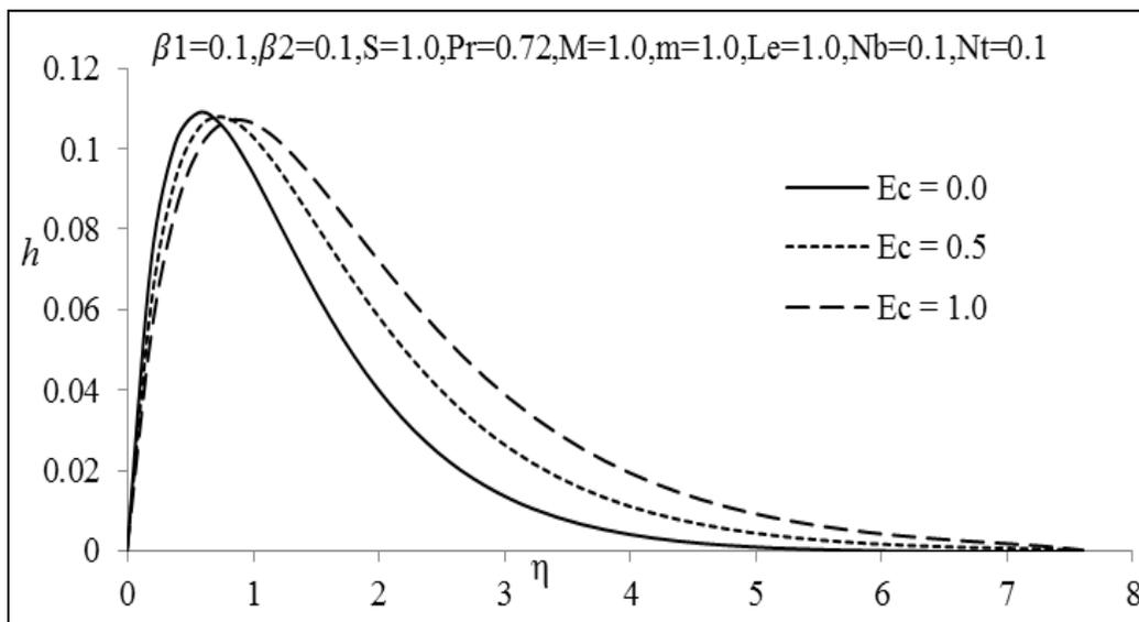
Fig 3(b): Transverse velocity profiles for various values of  $Ec$
