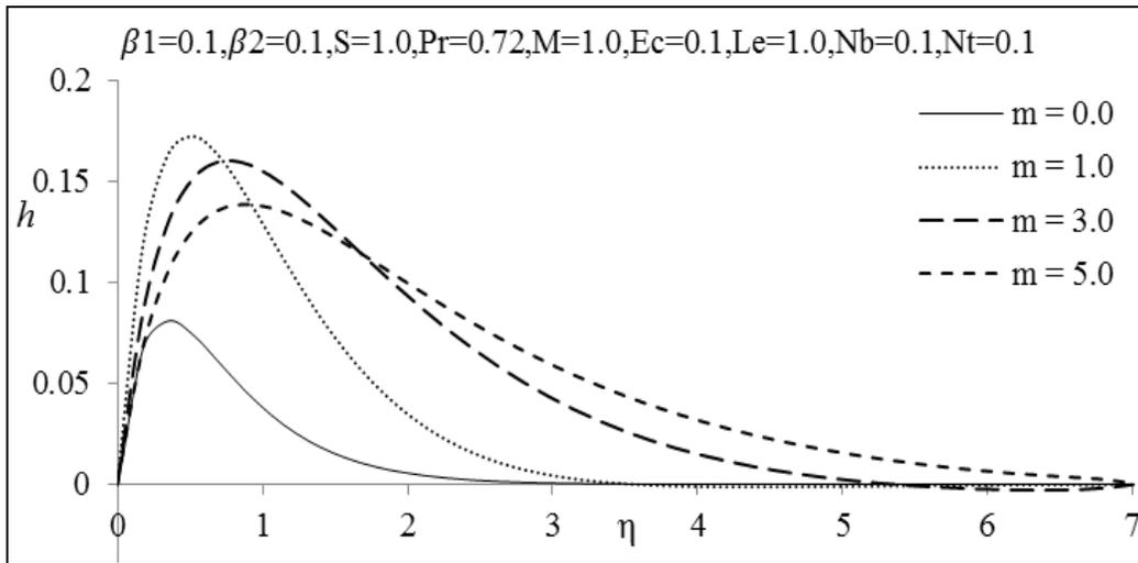
Fig 2(b): Transverse velocity profile for various values of m
