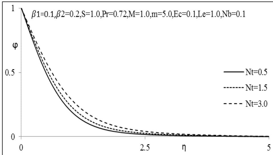
Fig 7(b): Concentration profiles for various values of  $Nt$
