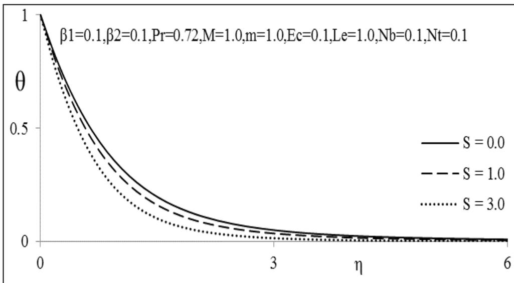
**Fig 5(c):** Temperature profiles for various values of  $S$
