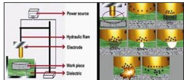
**Fig 1:** Spark Erosion Machining Unit
