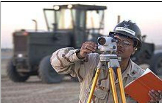
Fig 1: Surveyor at work with a leveling instrument
