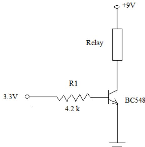
**Fig 3:** Actuating Module
